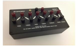
The RS1 is a cost efficient resistance Standard, intended e.g. for use in laboratory, research, metrology and educational applications where a precise yet economical resistance Standard is needed.
